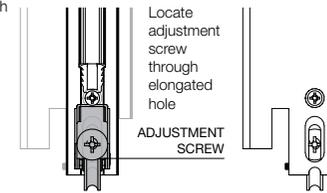
Rotate clockwise to raise the panel, counter-clockwise to lower the panel
