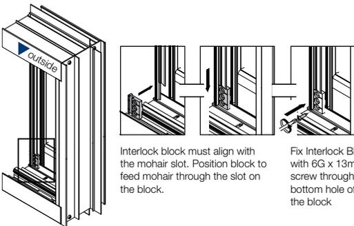
Interlock block must align with the mohair slot. Position block to feed mohair through the slot on the block.
