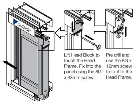
Lift Head Block to touch the Head Frame. Fix into the panel using the 8G x 12mm screw to fix it to the Head Frame.
