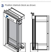
Interlock block must align with the mohair slot. Position block to feed mohair through the slot on the block.
