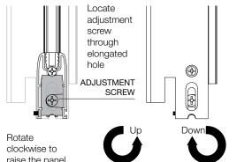
Rotate clockwise to raise the panel, counterclockwise to lower the panel
