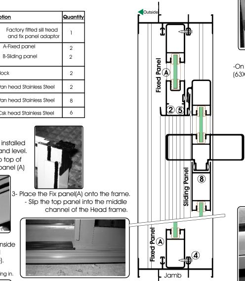
4 - On the inside, place screws (20x6) along the Jamb, approx. 500mm from top and bottom, between the mohair to fix panel to the Jamb.
