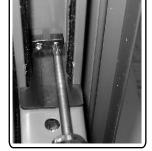
5-On top of the interlock, lift the Top fix block to touch the Head frame.
