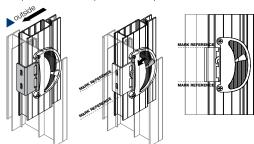
3 Open the door and place the keeper in position and secure into place using the 13mm pan head screws provided. Keeper can be adjusted.
