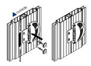
4 Mark and pre-drill holes as indicated and secure internal pull handle using the 13mm countersunk screws provided.
