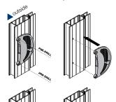
Close the door with the keeper, engage the keeper in the closed position and mark the position of the keeper.
