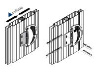
Place the keeper in position and secure into place using the 13mm pan head screws provided. Keeper can be adjusted.
