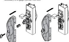
Secure cover with cover fixing screws.
