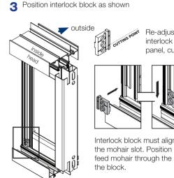
Re-adjust roller (Step 1) before fitting interlock block to the centre sliding panel, cut back block as shown Interlock block must align with Fix Interlock Block the mohair slot. Position block to with 6G x 13mm feed mohair through the slot on screw through the centre hole of the block.
