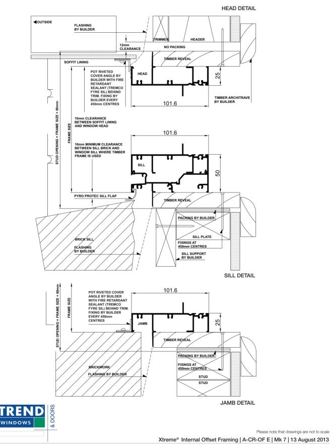
Xtreme® Internal Offset Framing | Building In Detail | Brick Veneer - 230mm wall
